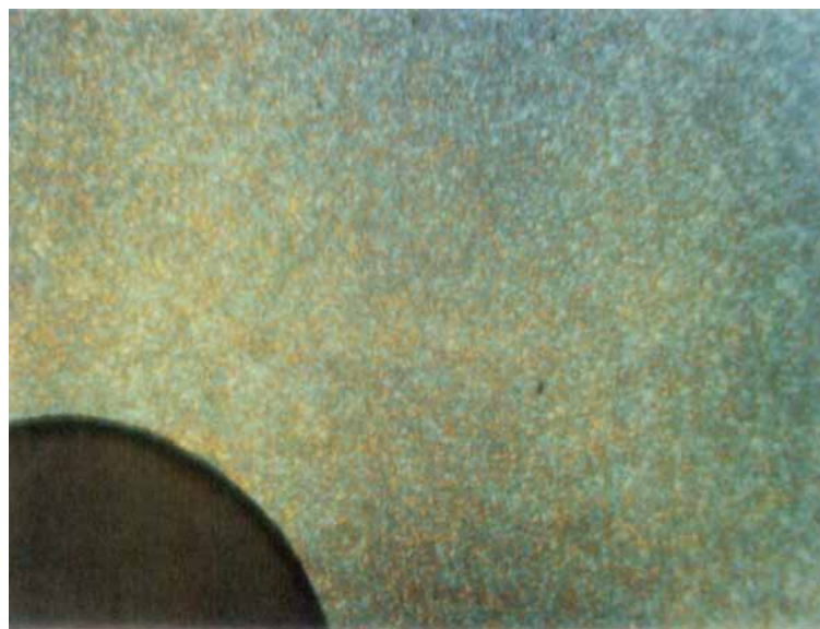
Figure 1. Polarizing optical micrograph of polymer 5 ( \times 100 magnification) in the smectic phase at 92^{\circ}\text{C} .
